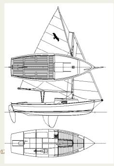
The GRP boat is made up of 12mm (½in) closed-cell foam sandwiched by layers of quadraxial glass cloth soaked in vinylester resin on the outside with a single layer on the inside. The transverse rigidity comes from the 9mm (23/64in) marine ply bulkheads.
