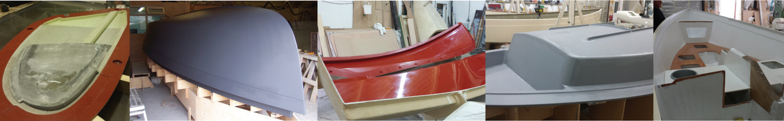
Below: stages in the building of Kite 3: from left: the NACA sectioned centreboard with its 80kg of lead ballast; the finished hull plug; the mould; hull and topsides about to meet; internal fit-out taking shape
